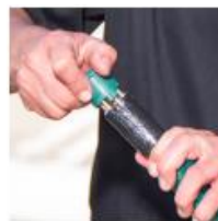
QCP (QUICK CHANGE PLUG) WITH CABLE GUARD
