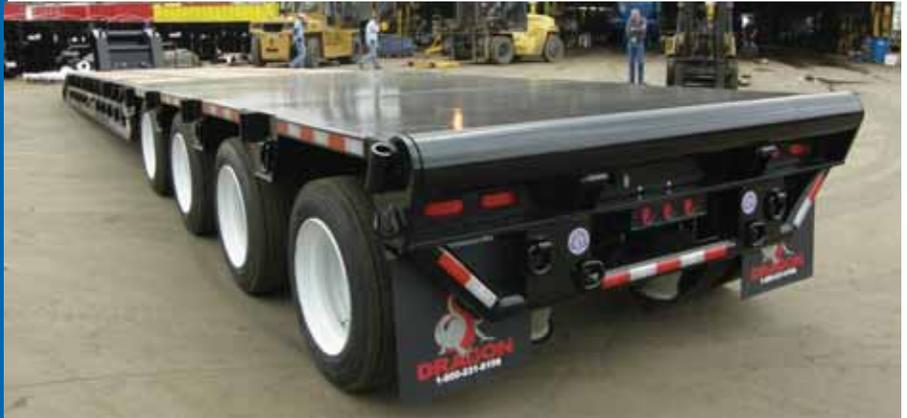
**Suspension:** 30,000 lb (per axle) air ride, air lift on front and rear axles, manual dump all axles, travel limit straps on all axles.
