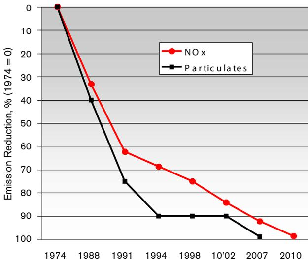
By 2010, diesel truck engines will have near-zero output of all regulated emissions.
